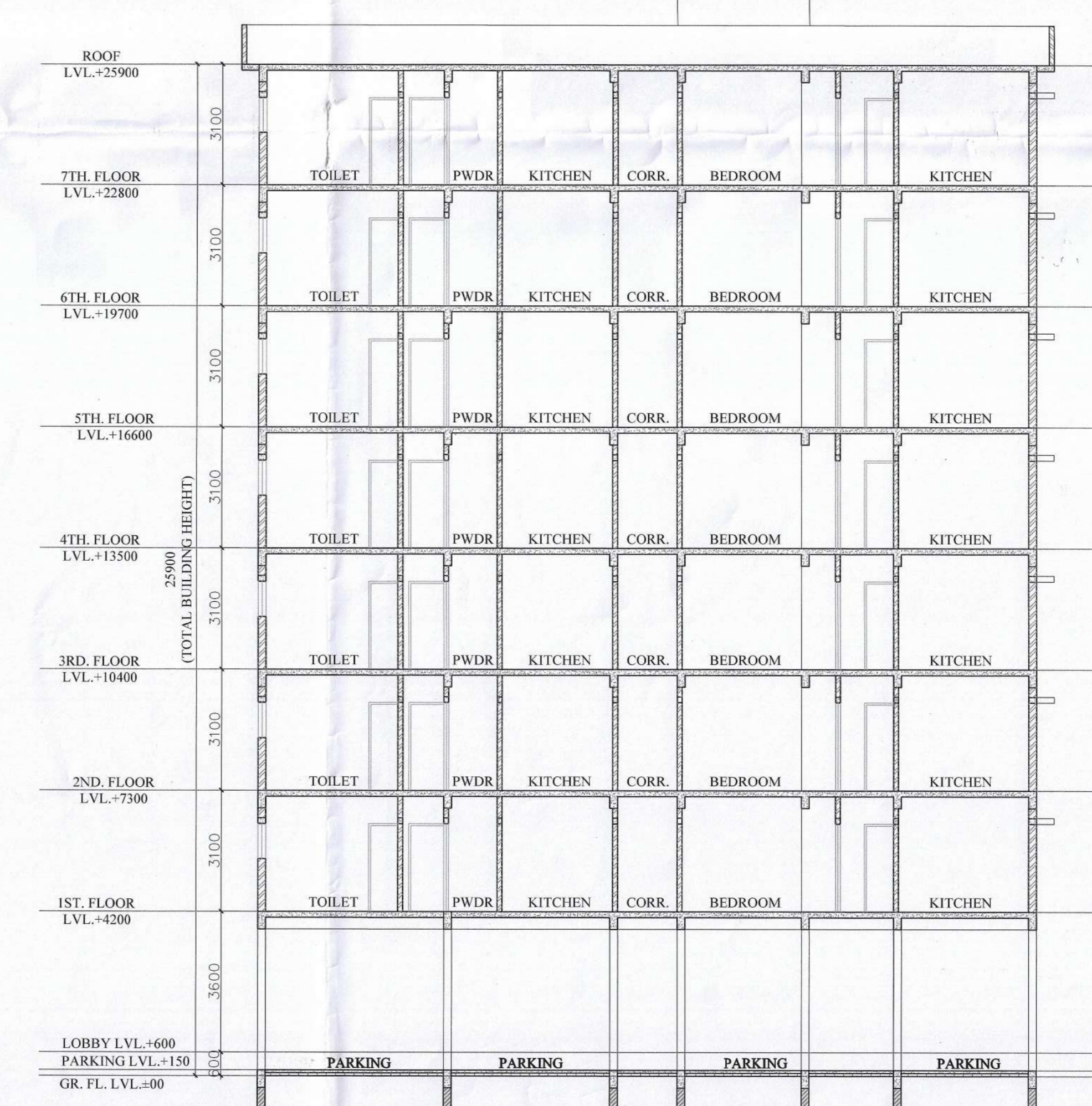
Y-Y THROUGH SECTION (BLOCK-2)
